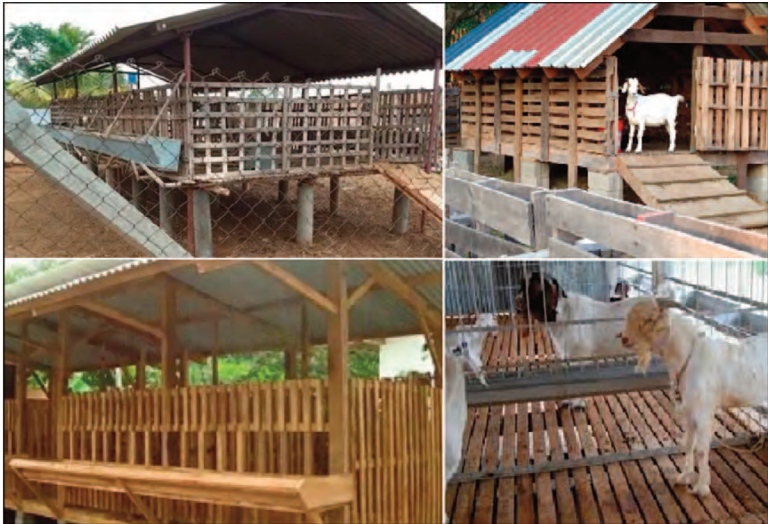
Figure 6.13 Raised floor with wooden walls, roof and feeding area goat pen
