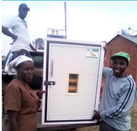
The installation of solar powered incubators has assisted farmers with easier access to hatching facilities at a lower price. Mechanical hatching over natural hatching has an advantage that it improves productivity in birds as hens quickly go back into laying as they do not need to spend time brooding the eggs.
