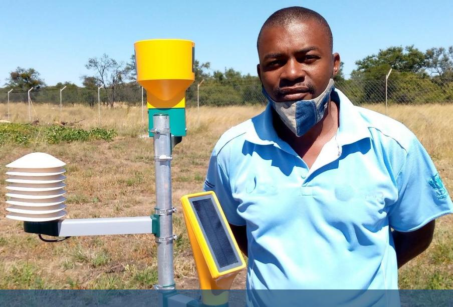
Solar powered smart weather stations at the ACEs to provide weather forecasts to farmers within a 40km radius of the stations. The stations automatically compile weather data and sends it to a portal where the responsible focal person can access and share with farmers. This will improve farmers' decision making for production.
